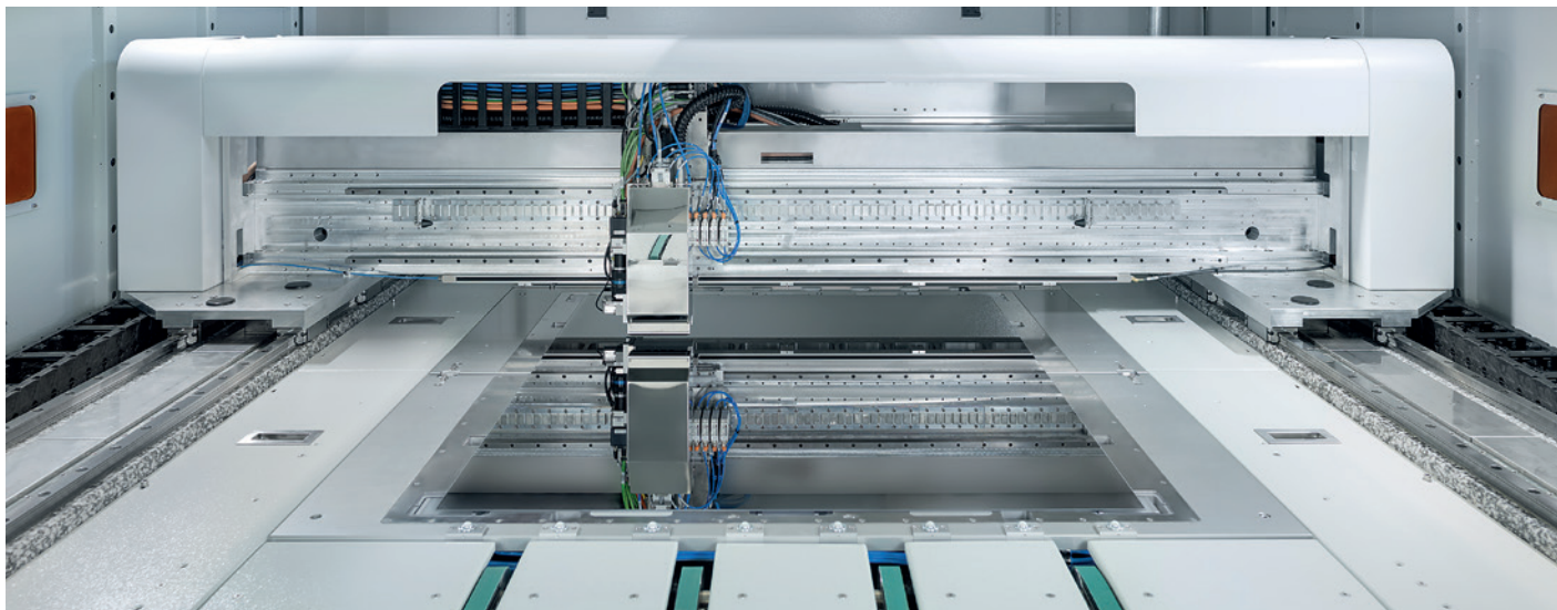
InnoLas Solutions is setting benchmarks in laser technology with its high-precision materials processing in the micro-range, including flat components up to 1.4 m x 2 m.
